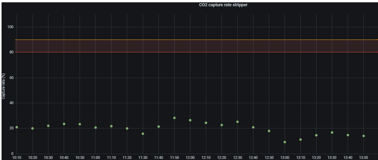
Figure 7 - Capture rate during STAR experiments (3M ammonia and 1M taurine) at 8 barg stripping pressure.
